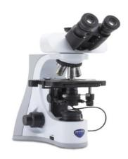
Trinocular darkfield microscope, 1000x, IOS W-PLAN objectives, for live blood analysis
